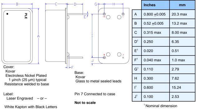
Pin **Function** Note 1 EFC 10 K ohm to ground –OR– 0.5 to 5.0V control voltage, depends on option ordered. Use the 30% value for initial operation 7 Ground (GND) 8 Output 14 Supply Voltage Recommend connecting appropriate power supply bypass capacitors as close as possible.  $(V_{cc})$
